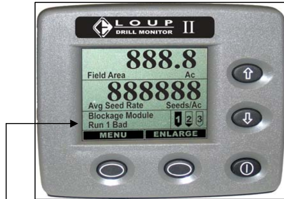
Acknowledged Run Bad alarm displayed in active alarm window
