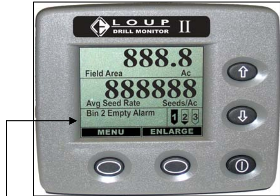
Acknowledged Empty Bin displayed in active alarm window
