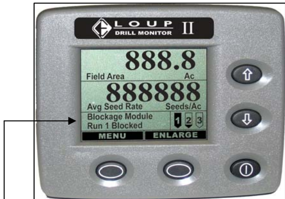
Acknowledged Run Blocked alarm displayed in active alarm window
