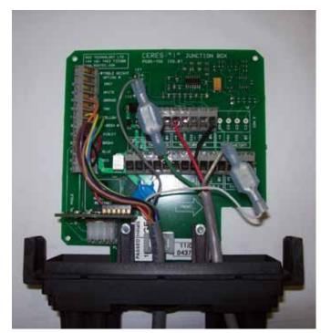
Connect the Green wire from the moisture sensor to the Gray wire from the Head Unit. Connect the Clear wire from the moisture sensor to the White wire from the head unit.
