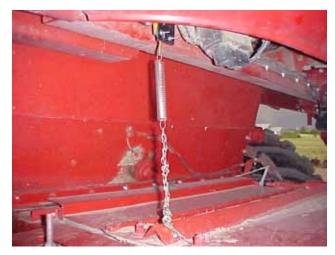
2. When attaching the chain to the feeder house, make sure a location is picked that will not be damaged by crop residue building up around the chain and sensor.
