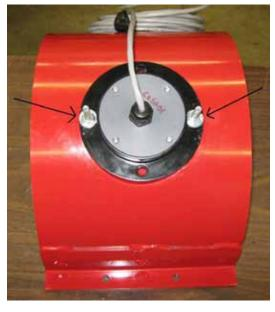
Use JB Weld Putty to blend the leading and trailing edge of the sensor to seal the sensor housing to the trap door to prevent grain leakage.
