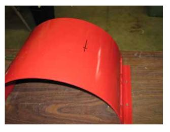
Cut a 3.25" hole **not** directly on the bottom. Locate the sensor towards the loaded paddle side of the elevator, towards the rear of the machine (about a 30-45 degree angle).
