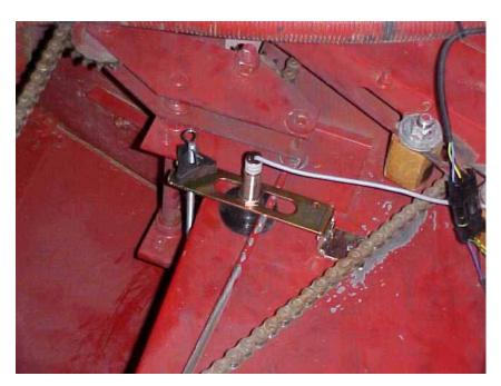
Once the yield sensor is positioned it may be necessary to modify the tensioning rod arrangement. This can be done by either moving the tensioning rod so that it does not interfere with the sensor or you can carefully grind one edge of the lens cover down as is shown in the picture above.
