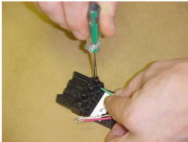
Once all wires are secured, press the cap onto the connector and plug into the mate on the monitor.
