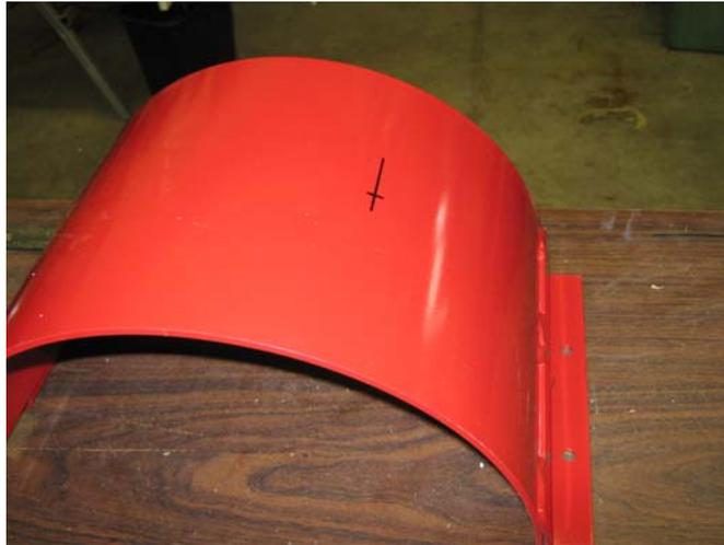
Cut a 3.25" hole **not** directly on the bottom. Locate the sensor towards the loaded paddle side of the elevator, towards the rear of the machine (about a 30-45 degree angle).
